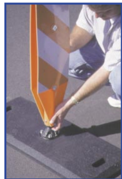
To unlock assembly simply pull keeper pin and rotate 90°
