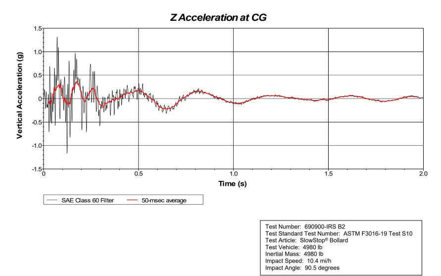
Figure F.5. Vehicle Vertical Accelerometer Trace for Test No. 690900-IRS B2 (Accelerometer Located near Center of Gravity
