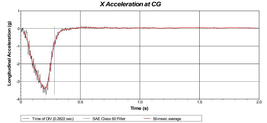
Test Number: 690900-IRS B2 Test Standard Test Number: ASTM F3016-19 Test S10 Test Article: SlowStop<sup>®</sup> Bollard Test Vehicle: 4980 lb Inertial Mass: 4980 lb Impact Speed: 10.4 mi/h Impact Angle: 90.5 degrees **F.3**.
