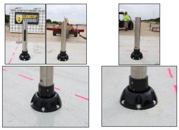
Figure 3.2. SlowStop® Bollard prior to Testing.
