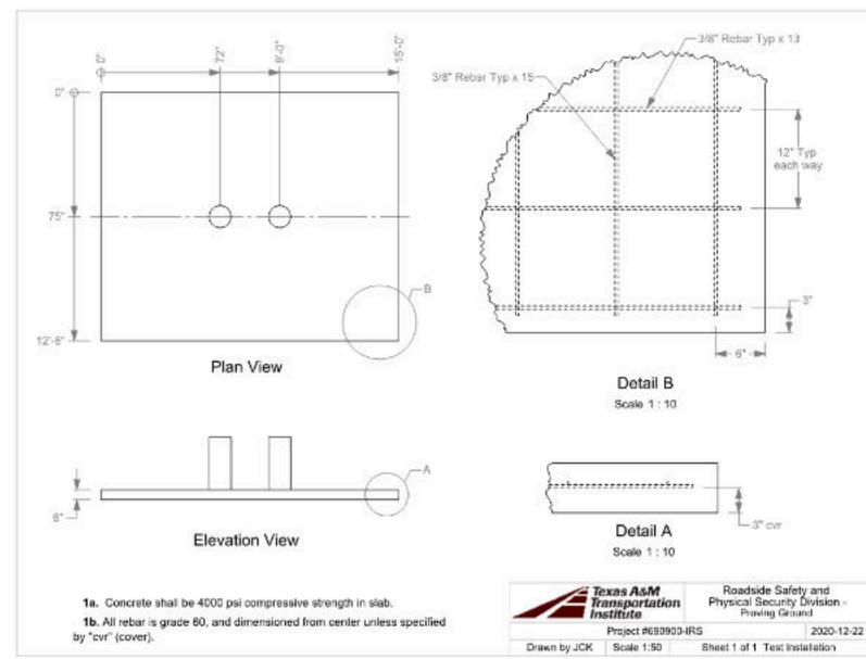
Figure 3.1. General Layout of SlowStop® Bollard.
