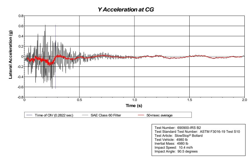
Figure F.4. Vehicle Lateral Accelerometer Trace for Test No. 690900-IRS B2 (Accelerometer Located near Center of Gravity).
