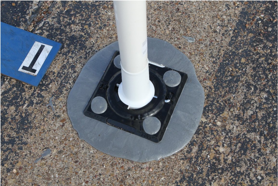
Figure B3. Delineators Attached to Concrete prior to Testing.
