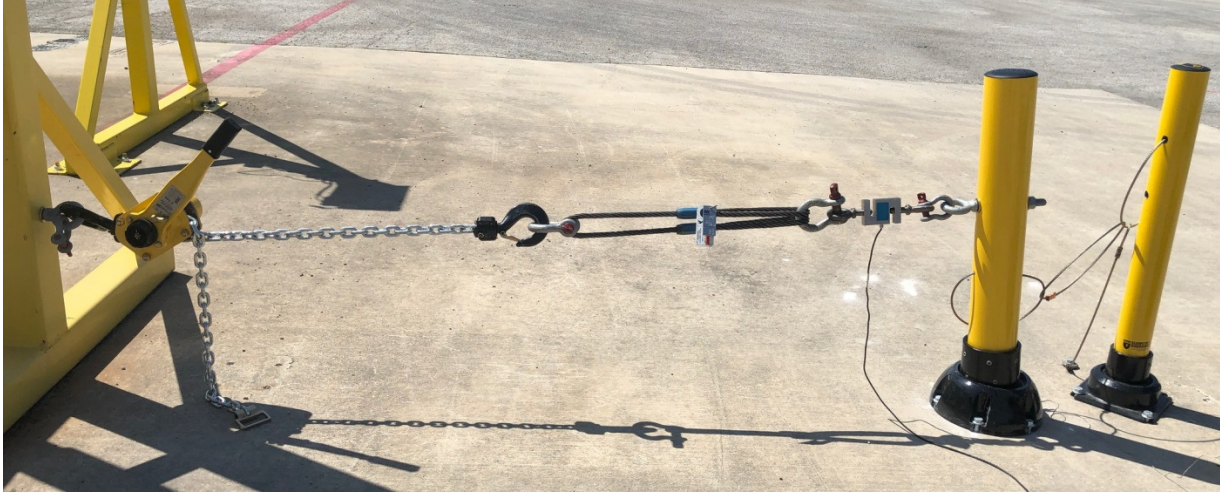
Figure 1 - Bollard Initial Condition
