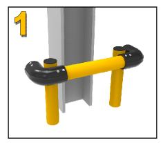
Your IronFlex column protector will arrive partially assembled. Place the assembled parts around the column (without bases). Be sure to carefully hold the pieces in place to prevent tipping. Check your drawing for orientation.
