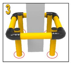
Mark the floor to create the center points for installation of the bases. Inspect for potential interferences such as steel plates and footers. Disassemble the frame to move it aside.
