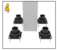
Install the four bases centered on the previous marks using the anchors provided. See our bollard installation instructions if you are unfamiliar with this step.
