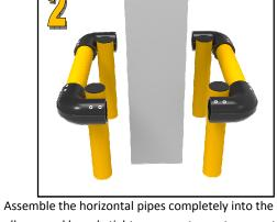
Assemble the horizontal pipes completely into the elbows and loosely tighten one or two set-screws to hold the complete frame in place.
